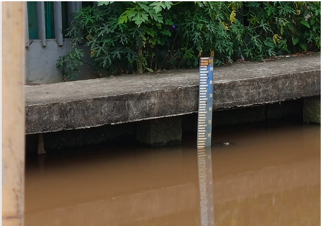
Photo 2. Measuring river depth: crucial data used to inform building codes and guide infrastructure adaptation in flood-prone areas, helping to mitigate potential damage.
